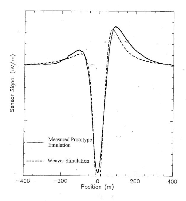
Figure 2 Comparison of Prototype SE Sweep with Weaver Simulation Prediction for 2000 ton Warship
