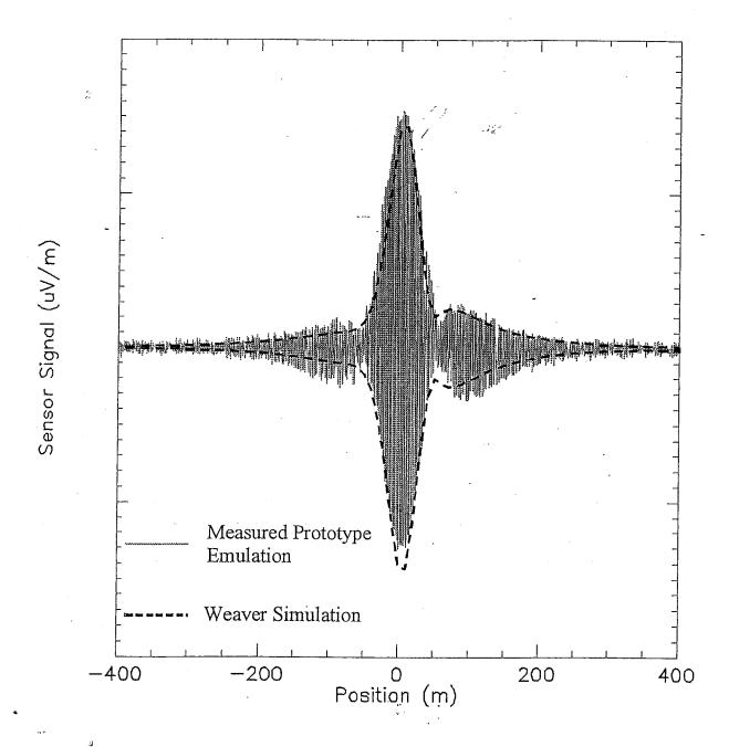
Figure 3 Comparison of Prototype AE Sweep with Weaver Simulation Prediction for 500 ton MCMV
