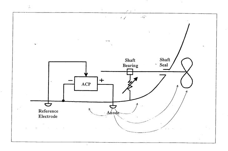
Figure 1 Active Cathodic Protection System
