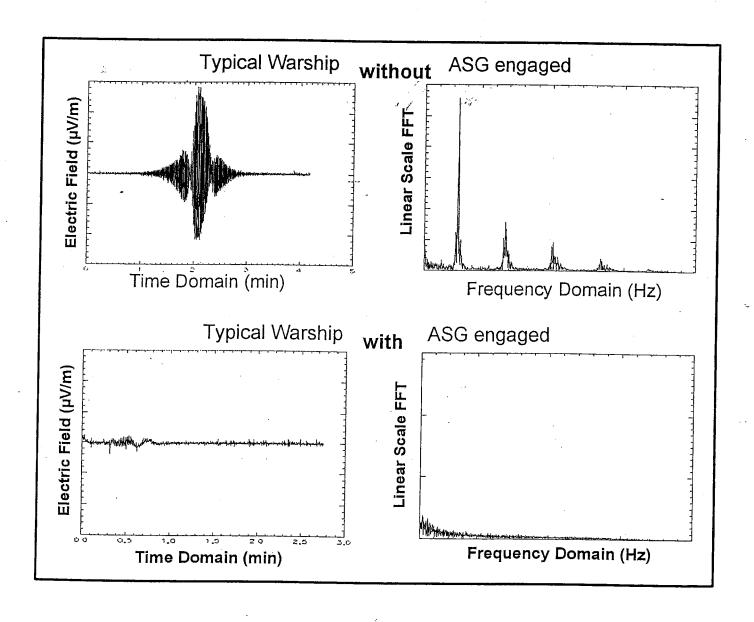
Figure 4 ASG Suppressed Electric siganture of Warship on Longitudinal Axis in Time and Frequency Domains
